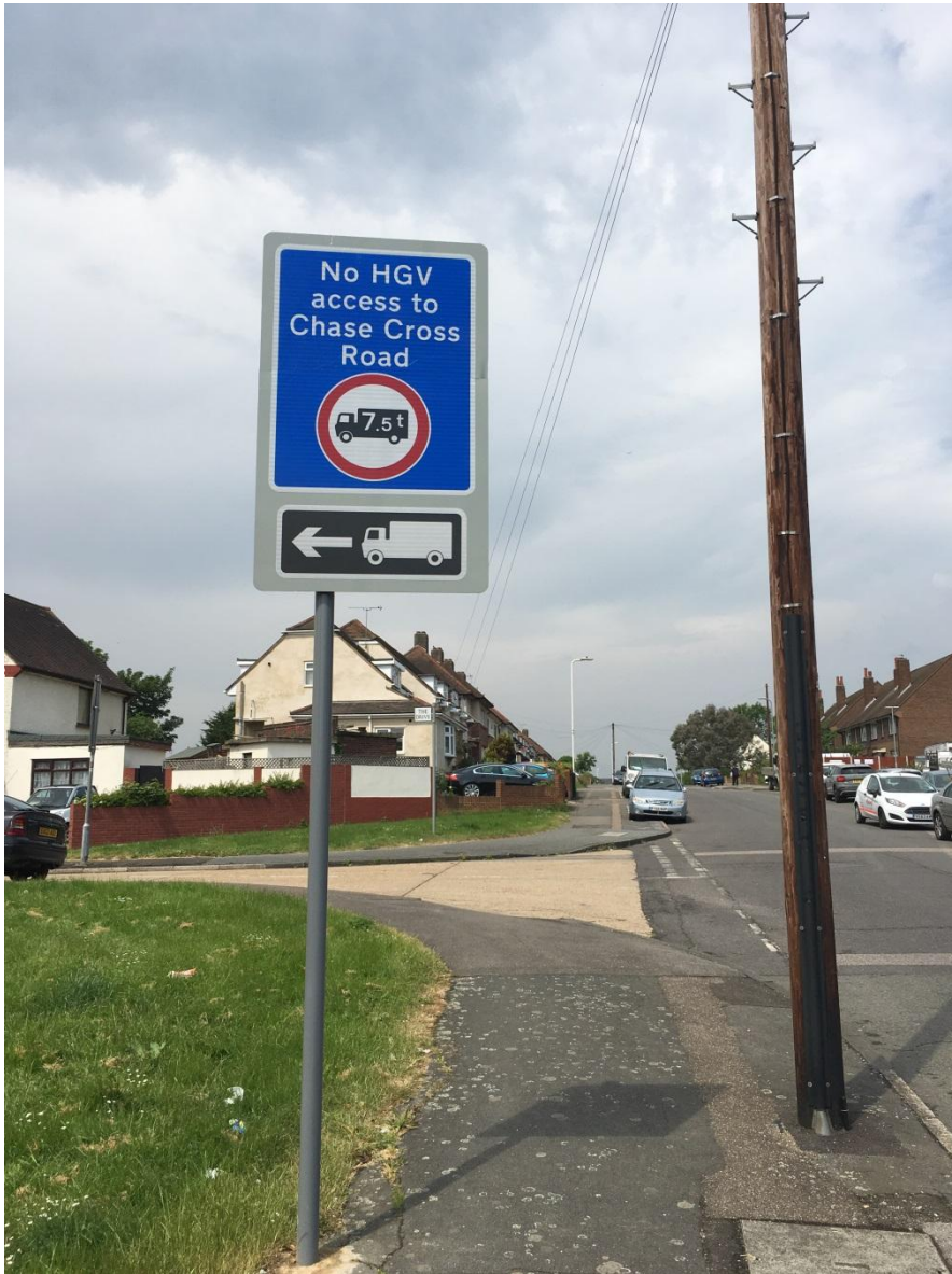
Example of advanced warning sign with lorry 'escape' route positively signed
